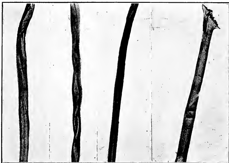
Figs. 7 and 8.—Micrographs of Cotton Fibres : (a) unripe fibre, (b) ripe fibre, (c) mercerized fibre. Micrograph of Silk Fibre : (d) illustrates the twofold character of the silk fibre and the splitting and expansion of the fibrils which occur in some Tussah Silks.
